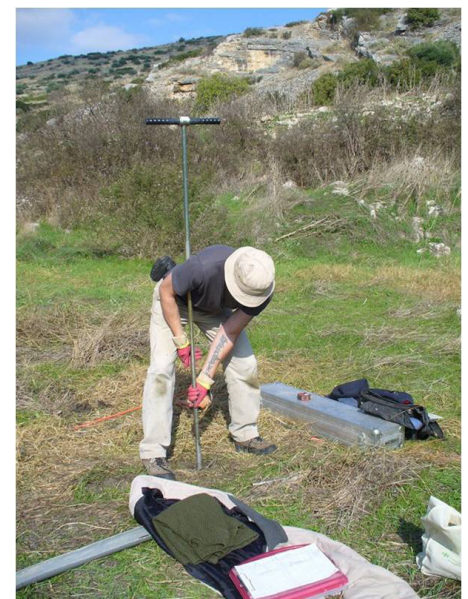
AROURA: Co-Director Michael Lane uses a soil auger to explore sediment deposition at the mouth of the Vrystika Katavothra sinkhole.
