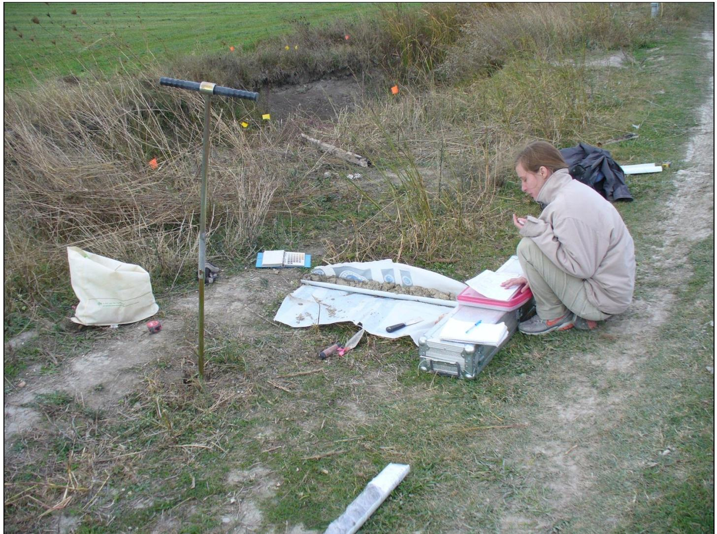
**Fig. 6.** Employment of soil-auger in Area I. Soil has been placed stratigraphically in PVC tray in center. E.V. Iliopoulou takes notes
