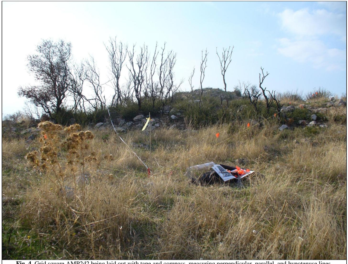
**Fig. 4.** Grid square AMP2d2 being laid out with tape and compass, measuring perpendicular, parallel, and hypotenuse lines.
