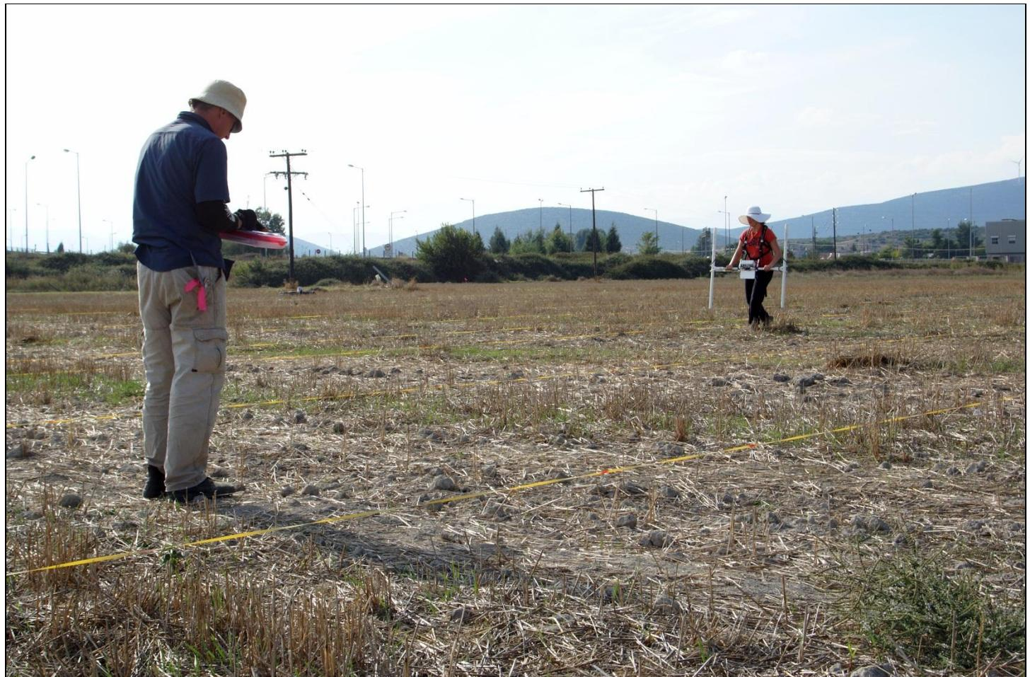
**Fig. 5.** Bloc of six grid squares demarcated with plastic strapping in Transect A1. M.F. Lane takes notes at L, while A.E. Cuneo operates Bartington 601-2 dual fluxgate gradiometer (magnetometer) at R (photograph by W.S. Bittner).
