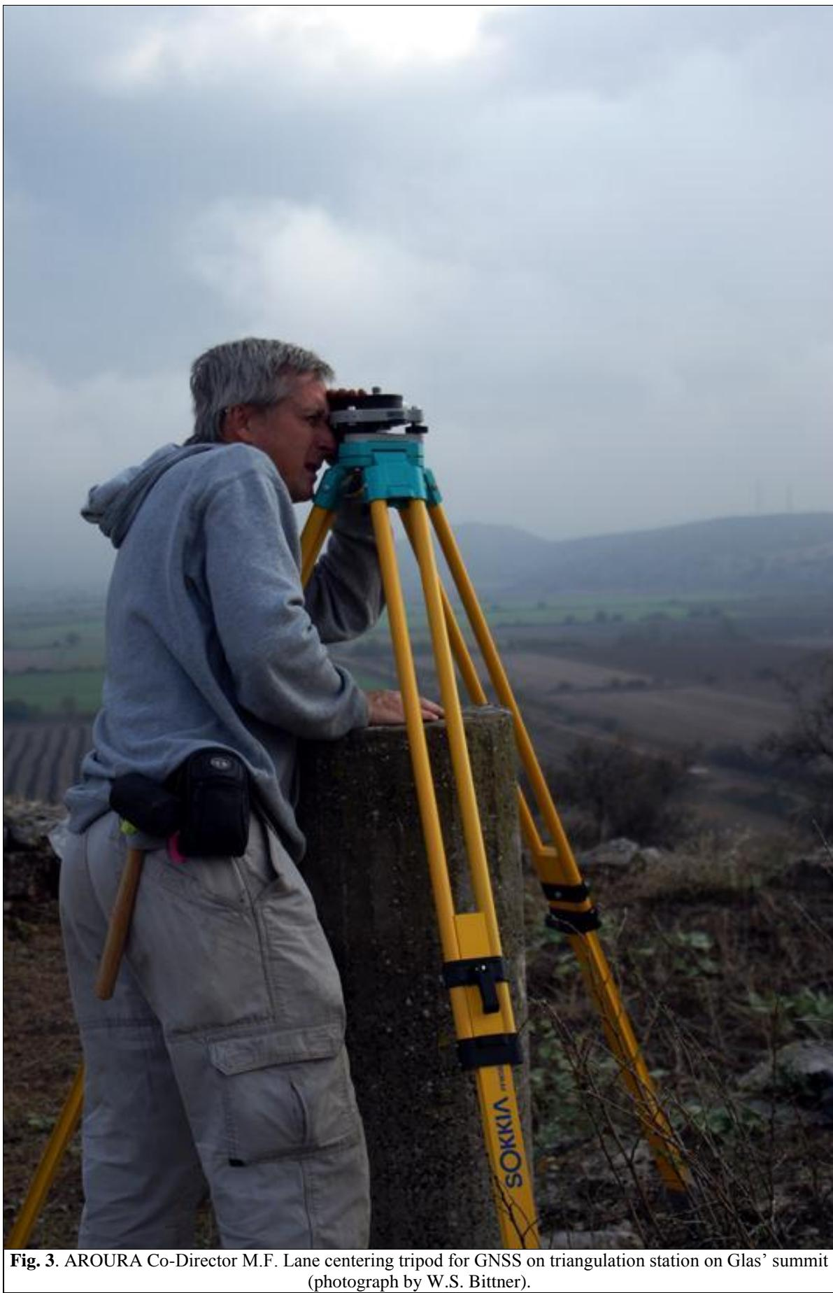
**Fig. 3.** AROURA Co-Director M.F. Lane centering tripod for GNSS on triangulation station on Glas' summit (photograph by W.S. Bittner).
