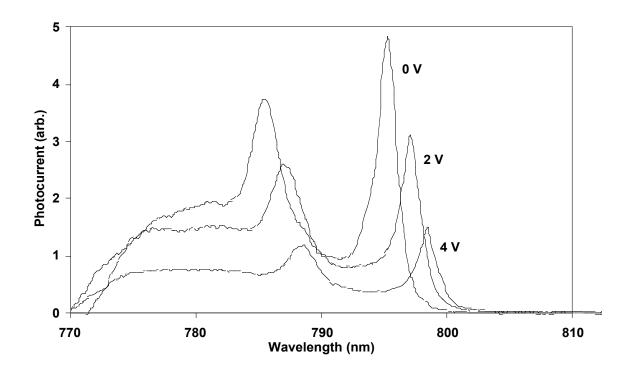
Photocurrent measured at 50 K on a 50-period quantum-well detector structure for three reverse-bias voltages. Exciton absorption features for both the heavy-hole and light-hole bands are present at this temperature.
