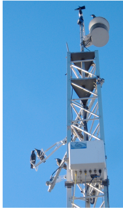
Figure 7. Birds roosting in the pathway of the sonic anemometer.
