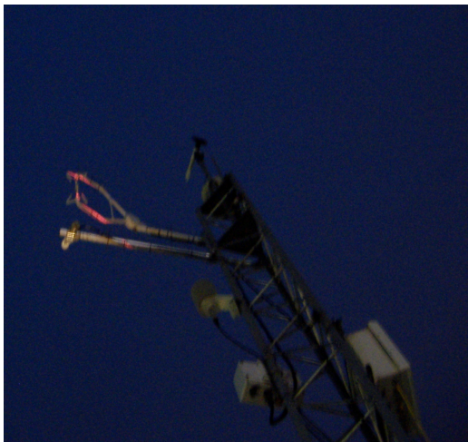
Figure 8. Using a laser level to determine the azimuth of the sonic anemometer.
