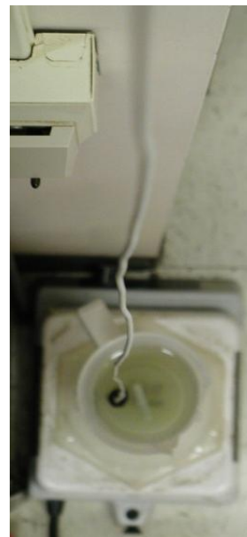
Figure 13. The sensor element of an Odyssey probe retains its coiled memory and any additional kinks that could cause measurement error if in contact with the well casing.
