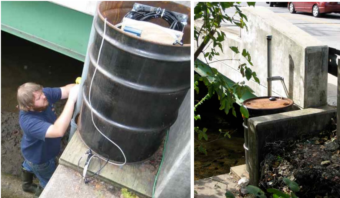
Figure 14. 55-gallon drum that can be used as an enclosure for the sensor package (a) with lid off; (b) secured.
