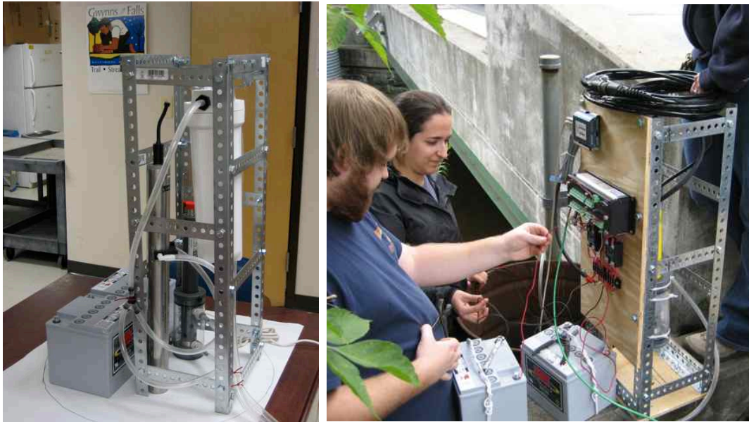
Figure 15. Cage constructed to hold sensor package inside 55-gallon drum.
