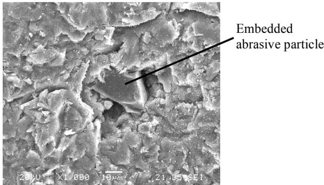
a) A micrograph of the treated surface
