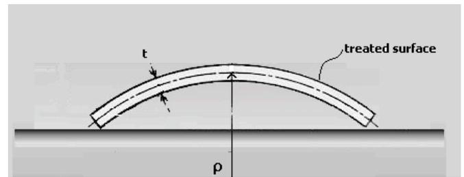
**Figure 3:** Schematic diagram of beam deflection and pertinent variables.
