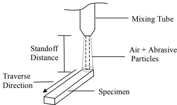
**Figure 2:** Details of the surface treatment process.
