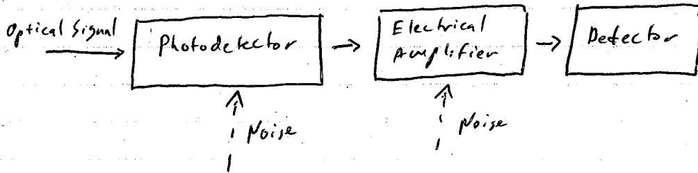
6. Fundamental sensitivity limit. Consider an ideal receiver (no noise), that can count even a single photon. No photons can arrive except in marks [no intersymbol interference (ISI)]. Quantum mechanically, the photon
