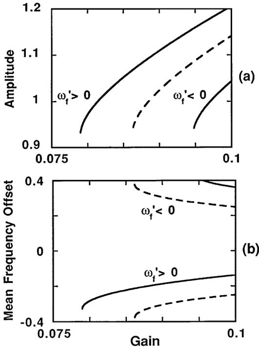
Fig. 1. Equilibrium values of (a) soliton amplitude  $A$  and (b) mean frequency offset from the filter frequency  $\Delta\omega$  versus excess gain  $\alpha$ , as determined from Eqs. (6) and (7). The filter parameters are  $\eta_2 = 0.1$ ,  $\eta_3 = 0.05$ , and  $|\omega_f'| = 0.44\eta_2$ . The dashed curves represent the equilibrium values ( $A^2, \omega$ ) for  $\eta_3 = 0$ .
