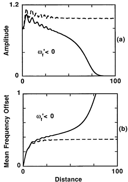
Fig. 2. (a) Soliton amplitude  $A$  (b) mean frequency offset from the filter frequency  $\Delta\omega$  as a function of distance  $z$  given in soliton periods, as determined by numerical solution of Eq. (2) with  $\omega_f' = -0.44\eta_2$ , corresponding to down-sliding. The solid curves correspond to the gain value  $\alpha_1$  given by Eq. (8), and the dashed curves correspond to  $\alpha_2$  given by Eq. (9).
