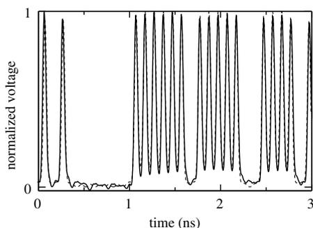
Fig. 3. The time sequence for a portion of the  $2^7 - 1$  PRBS pattern. The solid and dashed lines represent the measured and simulated time sequences, respectively.
