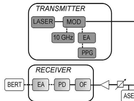
Fig. 1. Experimental setup. Solid lines correspond to optical signals and dashed lines correspond to electrical signals. OA: optical amplifier. OF: optical filter. PD: photodetector.
