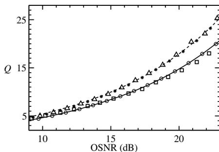
Fig. 2. The  $Q$ -factor as a function of the OSNR. The experimental data for the PRBS and 1010 patterns are shown with squares and triangles, respectively. The results obtained by combining the measured transmitter data with the receiver model are shown with circles and stars, and the simulation results with the transmitter-receiver model are shown with solid and dashed lines, respectively.
