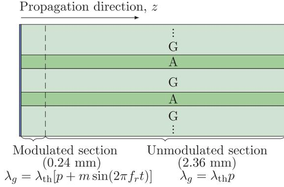
FIG. 1. Schematic illustration of an actively modelocked QCL with interleaved gain and absorbing periods. The labels G and A indicate gain and absorbing periods, respectively, and  $\lambda_g$  denotes the pumping strength.
