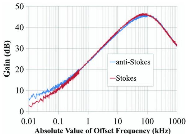
Fig. 2. Plots of the measured Rayleigh gain from a 10 km single-mode fiber with a 0 dBm incident laser beam.
