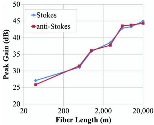
Fig. 5. Plots of the Stokes and anti-Stokes gain peaks versus fiber length for an 8 dBm incident laser beam.
