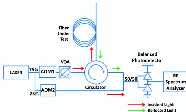
Fig. 1. Schematic diagram of our heterodyne interferometer. The acousto-optic modulators AOM1 and AOM2 are tuned to determine the IF.
