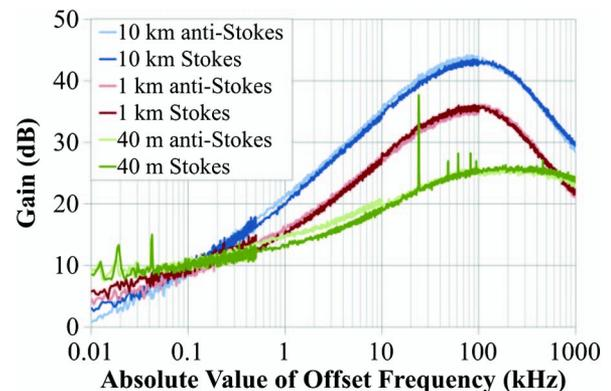
Fig. 4. Plots of the measured Rayleigh gain from 40 m, 1 km, and 10 km single-mode fibers with an 8 dBm incident laser beam.
