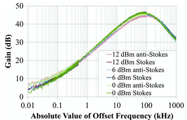
Fig. 3. Plots of the measured Rayleigh gain from a 10 km single-mode fiber for various incident power levels. The gain curves were normalized to the incident optical power.
