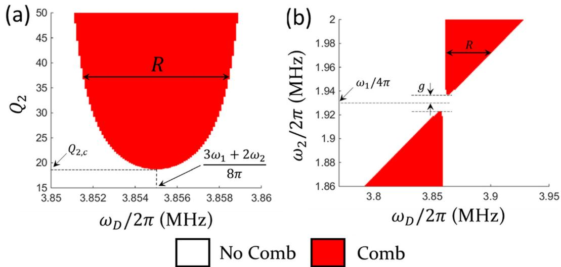
**FIG. 4.** Regions for generation of phononic frequency combs. (a) Quality factor of mode 2 vs drive frequency. (b) Resonance frequency of mode 2 vs drive frequency. System parameters: (a)  $\frac{\omega_1}{2\pi} = 3.86$  MHz,  $Q_1 = 4000$ , and  $\frac{\omega_2}{2\pi} = 1.92$  MHz and (b)  $\frac{\omega_1}{2\pi} = 3.86$  MHz,  $Q_1 = 4000$ ,  $Q_2 = 50$ .
