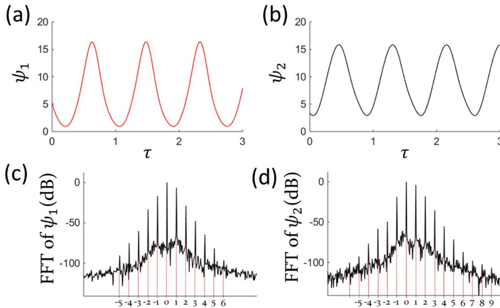
**FIG. 3.** Numerical simulation results for the mode amplitudes, Eqs. (5) and (6), within the phononic frequency comb boundary. Simulation parameters:  $\Delta_1 = 5$ ;  $\kappa = -9$ ;  $\Delta_2 = \frac{\Delta_1}{2} + \kappa$ ;  $\gamma_{21} = 1$ ;  $f = 20$ . (a) and (b) Time domain responses. (c) and (d) Corresponding fast Fourier transforms (FFT) showing the existence of phononic frequency combs.
