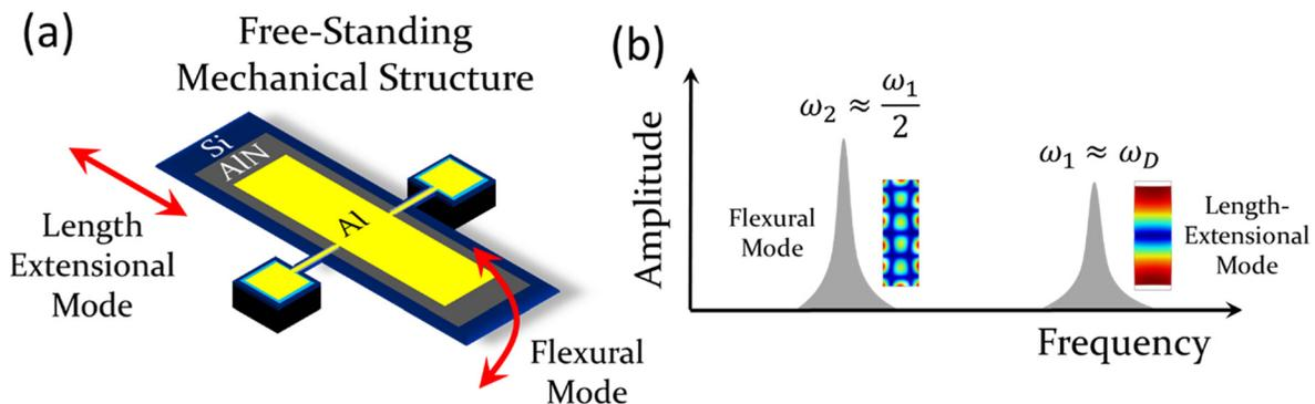
**FIG. 1.** Micromechanical resonator and phononic frequency comb concept. (a) Micromechanical resonator design used in Ref. 7 to generate phononic frequency combs. A length-extensional mode couples to a flexural mode through a nonlinear strain relationship. (b) Visual description of the mode coupling concept that results in phononic frequency combs, showing two modes where the resonance frequency of one mode is near double that of the other mode.
