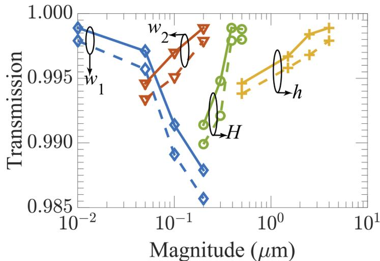
**Fig. 8.** The average transmission (solid lines) and minimum transmission (dashed lines) vs. each quantity's magnitude when varying  $w_1$  (blue diamonds),  $w_2$  (red triangles),  $h$  (yellow pluses), and  $H$  (green circles) for concave cone motheye structures under normal incidence with  $W_1 = 2w_2$  and  $W_2 = 0.60 \mu\text{m}$ .
