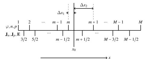
Gridding scheme used in device model for multilayer devices
