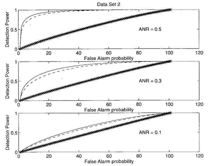
Fig. 9. ROC curves produced by SSC, TSC without bias, and TSC with bias, respectively, based on data set 2 with (a)  $\alpha_3/\sigma = 0.5$ , (b)  $\alpha_3/\sigma = 0.3$ , and (c)  $\alpha_3/\sigma = 0.1$ , where the asterisked, dotted, and solid curves are generated by SSC, TSC without bias, and TSC with bias, respectively.
