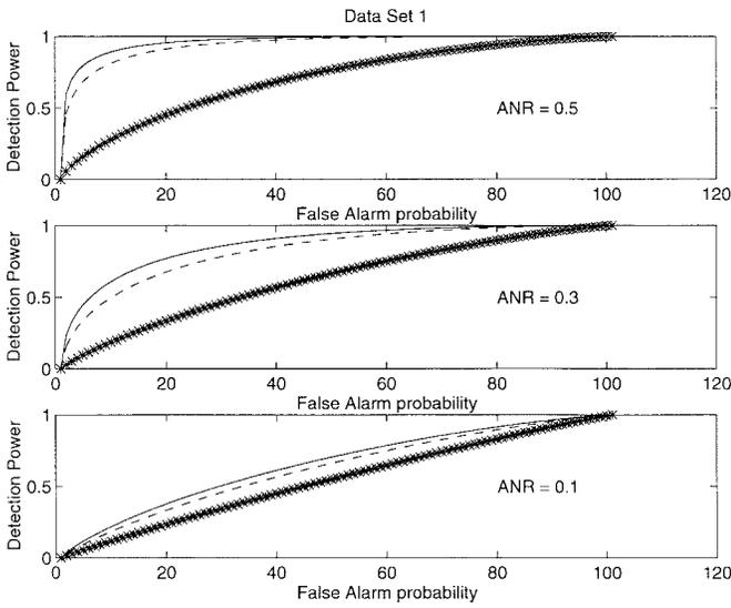
Fig. 8. ROC curves produced by SSC, TSC without bias, and TSC with bias, respectively, based on data set 1 with (a)  $\alpha_3/\sigma = 0.5$ , (b)  $\alpha_3/\sigma = 0.3$ , and (c)  $\alpha_3/\sigma = 0.1$ , where the asterisked, dotted, and solid curves are generated by SSC, TSC without bias, and TSC with bias, respectively.
