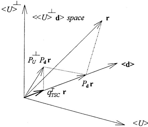
Fig. 2. Target signature space orthogonal projection classifier (TSC).
