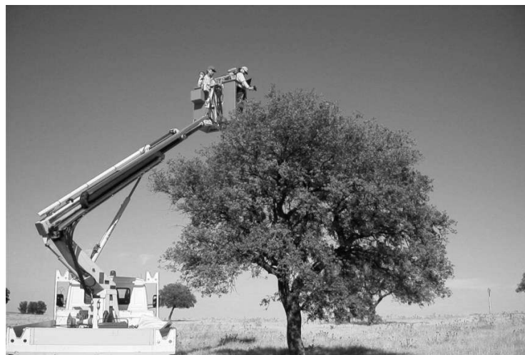
Figure 3. Ground-truth data collection at the top of C3 tree crown by using an ASD FieldSpec Pro spectroradiometer.
