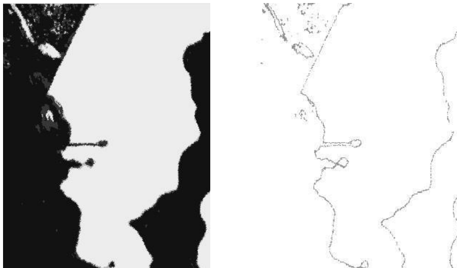
Figure 13. (Left) Guadiloba reservoir after SOM neural network classification, where the land is coloured in black and the water in very pale grey and light grey. (Right) Guadiloba reservoir scene, portraying only the class that could represent polluted water in the SOM neural network classification.
