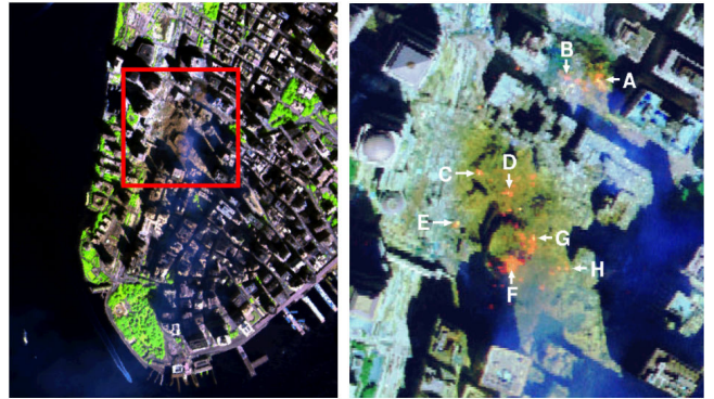
Fig. 2. Hyperspectral image (left). Location of fires in World Trade Center (right).
