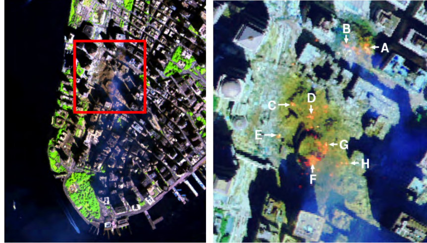
Figure 4. False color composition of an AVIRIS hyperspectral image collected by NASA's Jet Propulsion Laboratory over lower Manhattan on Sept. 16, 2001 (left). Location of thermal hot spots in the fires observed in World Trade Center area, available online: http://pubs.usgs.gov/of/2001/ofr-01-0429/hotspot.key.tgif.gif (right).
