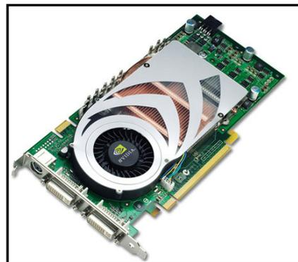
**Figure 9.** NVidia commodity graphic processing unit.
