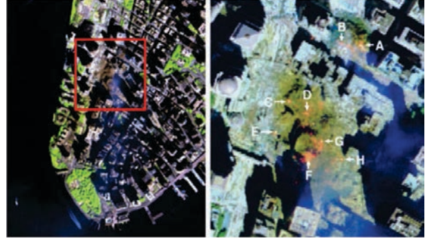
Fig. 3. False color composition of an AVIRIS hyperspectral image collected by NASA's Jet Propulsion Laboratory over lower Manhattan on 16 September 2001 (left). Location of thermal hot spot fires in World Trade Center area(right).
