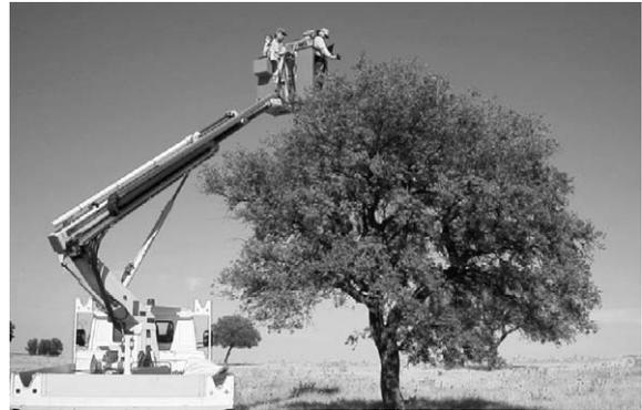
Fig. 7. Ground-truth data collection at a Dehesa test site in SW Spain by using an ASD FieldSpec Pro spectro-radiometer.
