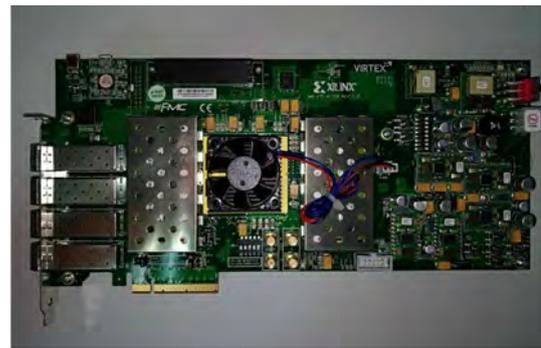
Fig. 4 Xilinx VC709 connectivity kit with a XC7VX690T-2FFG1761C FPGA
