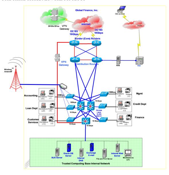
You are responsible for a corporate WAN spanning 10 remote facilities and interconnecting those facilities to the central data processing environment. Data is transmitted from a remote site through a VPN appliance situated in the border layer of the routing topology; the remote VPN connects to the internal Oracle database to update the customer data tables. Data transaction from the remote access to the corporate internal databases is not encrypted.
